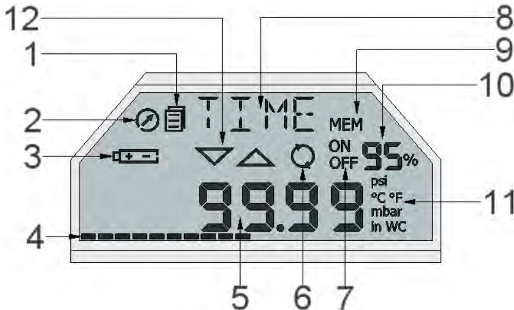
Figure 5: ESS3 display indications
