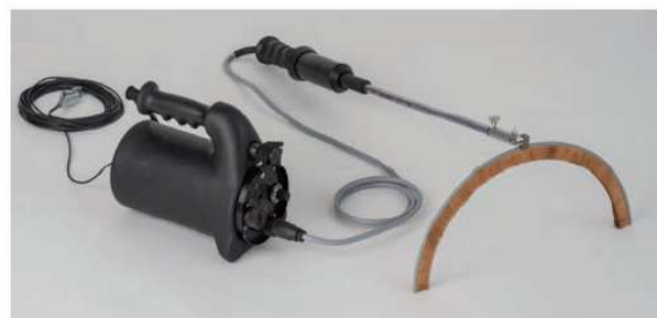
Figure 2: UNION Isolation Tester type V with semi-circular test brush
