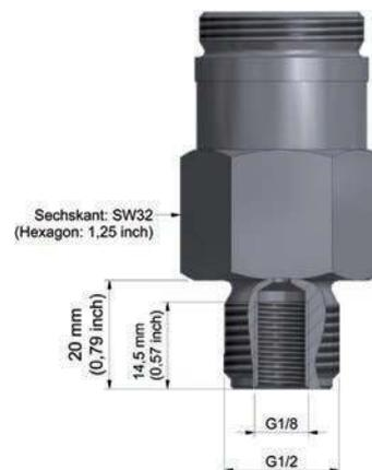
Figure 3: Pressure sensor
